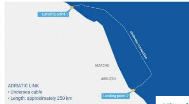
Figure 6 : Adriatic Link cable route. Credit: Terna S.p.A. [27]
