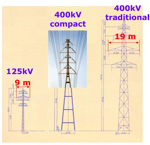
Steel lattice tower of 125kV-line and Swiss compact tower for 400kV/132kV-line as well as standard design
